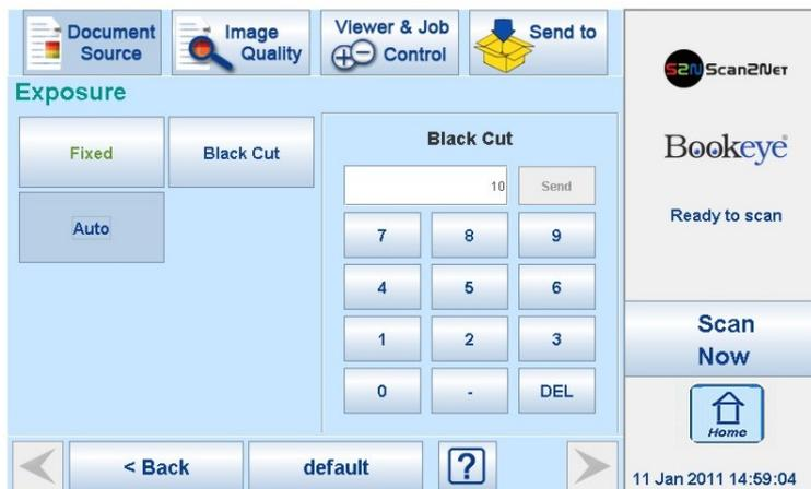
Picture 91: Numeric key pad to set threshold value
